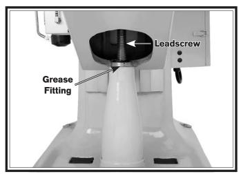
Figure 52. Table elevation leadscrew and grease fitting.
